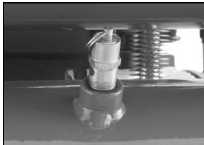
Figure 8. Safety drain valve.
